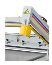
Emergency security bar with automatic reverse from descending to ensure operator safety in all machine area
